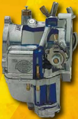
Accelerator Pump Cutaway
